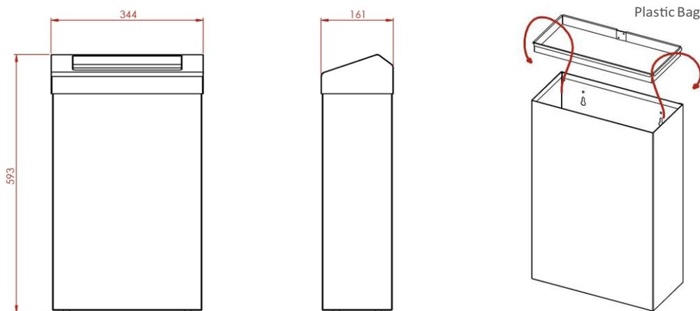
Height: 593mm Width: 344mm Depth: 161mm Weight: 6Kg Capacity: 30 Litre
