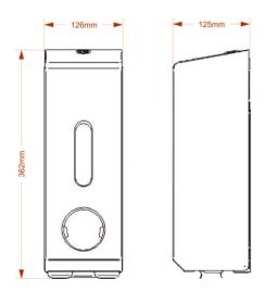
Height: 362mm Width: 126mm Depth: 125mm Weight: 1.9Kg Capacity: x3 Standard Toilet Rolls
