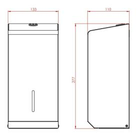
Height: 277mm Width: 133mm Depth: 110mm Weight: 1.3Kg Capacity: Approx x600 Sheets
