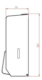
Height: 251mm Width: 108mm Depth: 91mm Weight: 1.2Kg Capacity: 900ml
