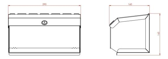
Height: 165mm Width: 290mm Depth: 160mm Weight: 1Kg Capacity: x1 10" Couch Roll
